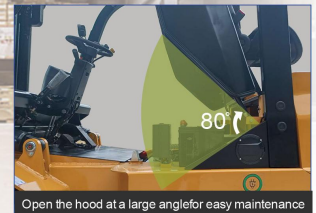
Open the hood at a large angle for easy maintenance
